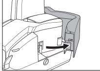
**2** While lowering the open lever, open the reading unit.
